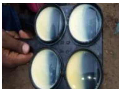
Figure 3. CMT paddle milk with reagent and gel formation.
