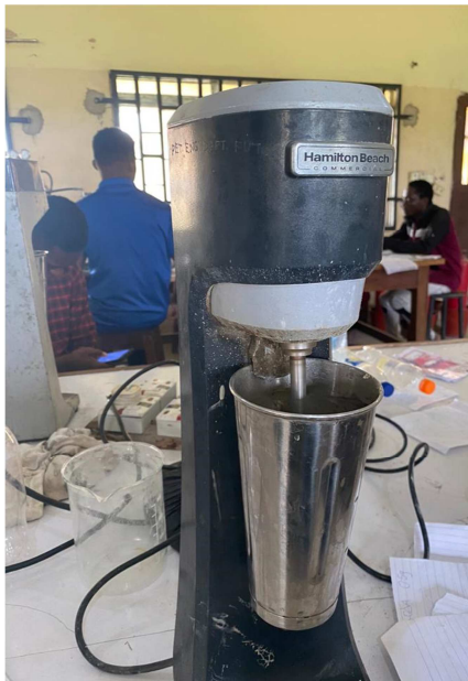
Figure 8. Hamilton beach mixer used to mix the sample concentration.
