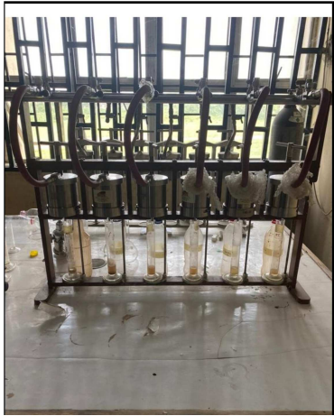
Figure 11. API filter press.
