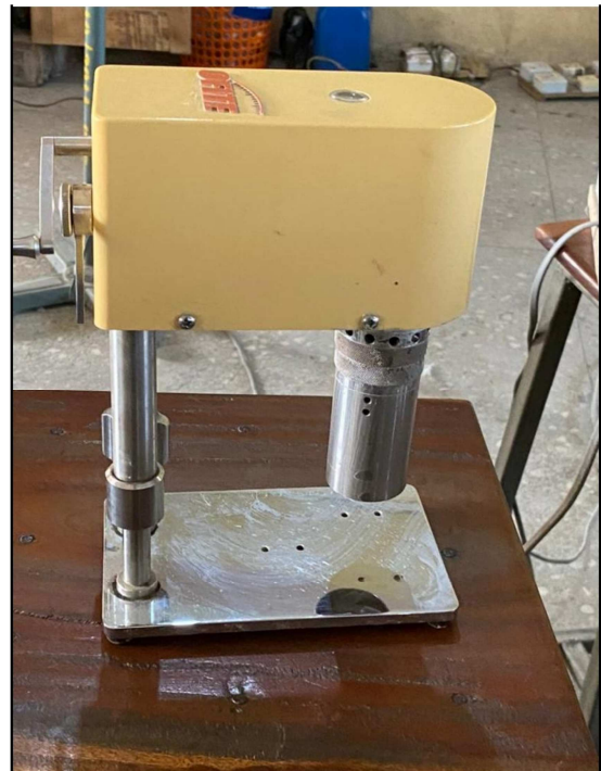
Figure 10. VG meter used to determine gel strength.
